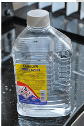
FIGURE 13.3.8 White spirit contains a mixture of alkanes. It is a useful solvent for other non-polar liquids.
