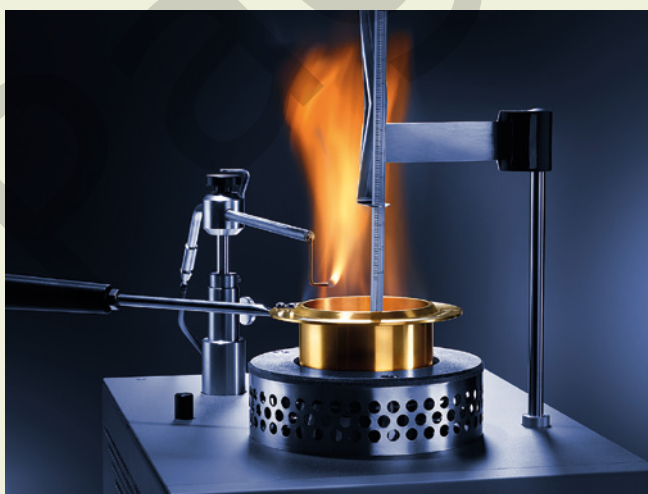
FIGURE 13.3.27 This apparatus measures the flashpoint of fuels. The fuel is heated steadily in a metal cup and, at intervals, a flame is brought above the liquid in the cup. The flashpoint is the lowest temperature at which the fuel will ignite when the flame is brought above it.
